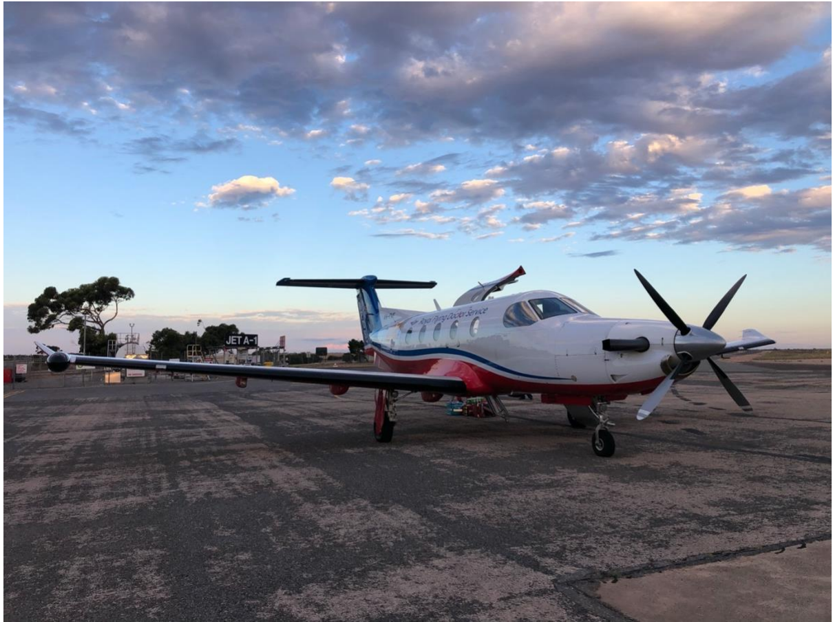
1 2 Figure 3. One of the RFDS Pilatus PC-12 turboprop aeroplanes used by MedSTAR to 3 respond to cases beyond a 200-kilometre radius of Adelaide.
